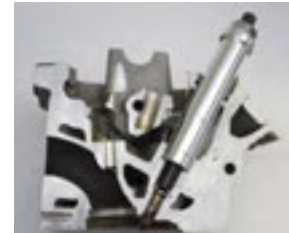
PULLING BROKEN PLUG
