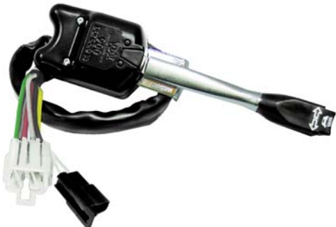
vsm915Y103 Replacement Turn Signal Switch for: KENWORTH K301D230;18500D044 • 8 wire harness • Handle features built-in push button high/low beam selector switch • 16 bulb capacity for hazard warning • 8 bulbs per side for turn signal flashing
