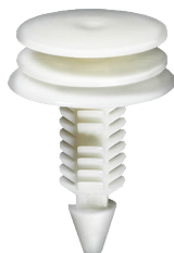
19270 (10285935) White Nylon Trim Panel Retainer Overall Length: 1-3/16" Buick Century & Regal, Chevrolet Venture, GM Truck Express/Savana, Olds Silhouette & Pontiac Trans Sport 1997 - On
