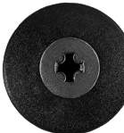
17081 (91524-SE0-003) Black Nylon Cowl Push-Type Retainer Head Diameter: 18mm Stem Length: 12mm Fits into 6mm Hole Accord 1986-On
