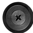
14698 (90688-SB0-003) Black Nylon Push-Type Retainer Head Diameter: 18mm Stem Length: 11mm Fits into 6mm Hole
