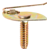
19626 (Ford: 358560; Chry: 1560058, 6010029; GM: 568792, 574355, 1165051) Moulding Fastener Bolt: #10-24 x 3/4" Plate Length: 1" Plate Width: 1/2"
