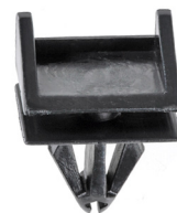
21504 (GM: 10445899) Black Nylon Door Moulding Clip Top Head Size: 14mm x 20mm Bottom Head Size: 15.5mm x 20mm Stem Length: 14mm Fits into 9mm Hole GM SUV's 1997 - On
