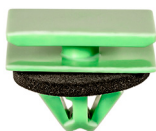
21504 (GM: 10445899) Black Nylon Door Moulding Clip Top Head Size: 14mm x 20mm Bottom Head Size: 15.5mm x 20mm Stem Length: 14mm Fits into 9mm Hole GM SUV's 1997 - On
