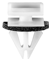
20353 (10442914) White Nylon Rocker Panel Moulding Clip Top Head Size: 1/2" x 9/16" Bottom Head Size: 9/16" x 5/8" Stem Length: 9/16" Fits into 7/16" Hole Buick Rendezvous 2002 - On
